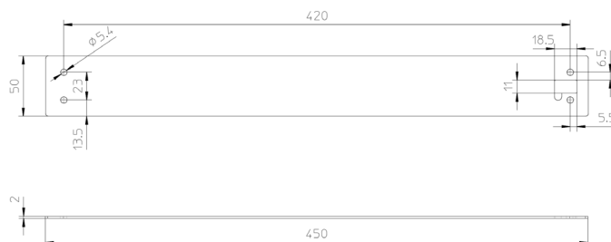
Dimensions PK00578 (VBlech 400) Material Stainless steel
