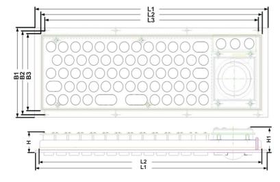
L1 = 315,00mm L2 = 299,00mm 288,00mm B1 = 115,00mm B2 = 109,00mm B3 = 99,00mm 27,55mm 32,75mm H2 = 21,50mm H3 = 3,00mm H4 =3,50mm
